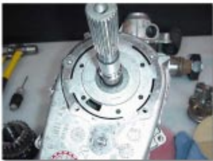
(Fig. 10) Oil Pump Removal
