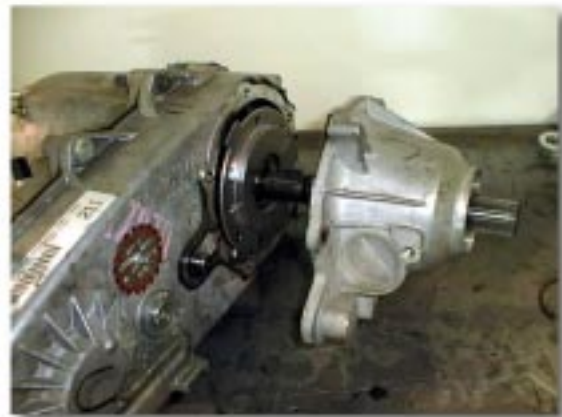
(Fig. 8) Rear Tailhousing Removal
